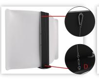
10. Place the cable on the (C) via a hook on the end of the cable, and on the bottom use(D) to hook and tension, screw tension hook till the frame with the TV is 90°.
