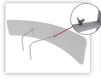
13. Slide the hanging post on to the header and tighten the bolts on to the small shaft.
