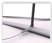
7. Place the black vertical shafts in the bottom ring.
