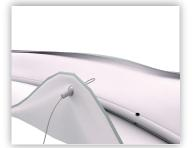
6. Thread cable support through eyelet.
