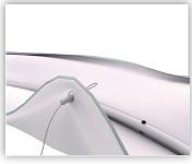
6. Thread cable support through eyelet.
