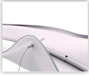
6. Thread cable support through eyelet.
