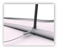
Place the black vertical shafts in the bottom ring.
