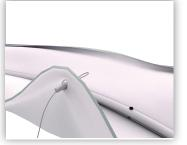
Thread cable support through eyelet.
